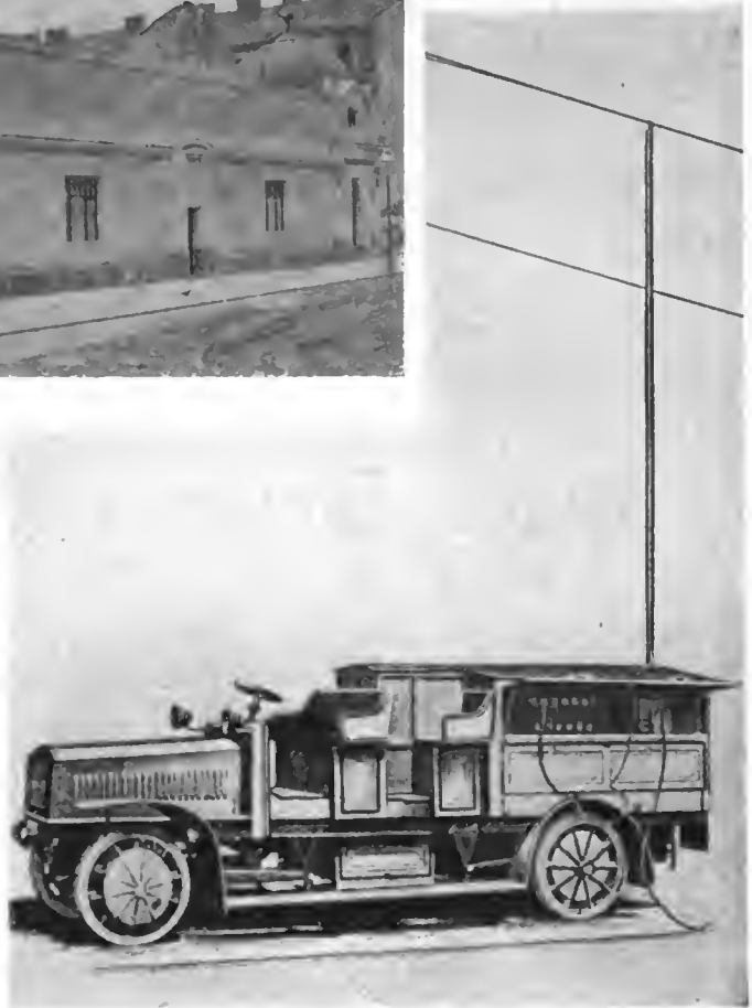
The 3-ton electric used by the Great Berlin Tramways for repair work. It may be charged from the trolley, as illustrated
